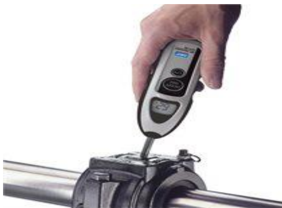
Slika 23. Mjerenje temperature ležaja pomoću kontaktnog termometra (Izvor: http://www.skf.com/my/products/condition-monitoring/basic-condition-monitoring-products/thermometers/general-purpose-thermometer/index.html )
