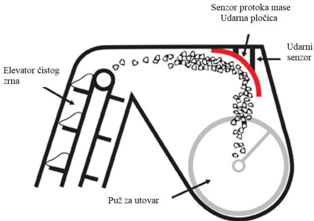
Slika 2. Prikaz udarnog senzora (Izvor: <https://www.farm-equipment.com> )
