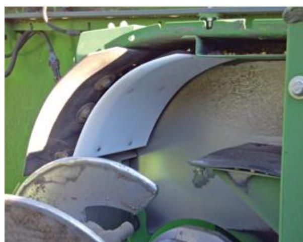
Slika 3. John Deere udarni senzor (Izvor: <https://www.maywes.com/products/mass-seed-flow-sensor-impact-plate-8-1-4-x-12-1-2-x-1-8-thick-kit> )
