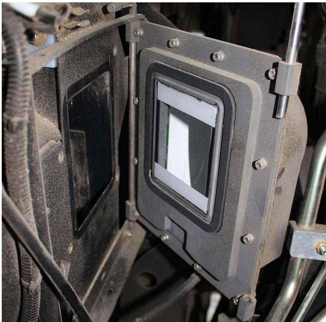
Slika 5. Optički senzor čistog zrna (Izvor: <https://www.fwi.co.uk/machinery/harvest-equipment> )
