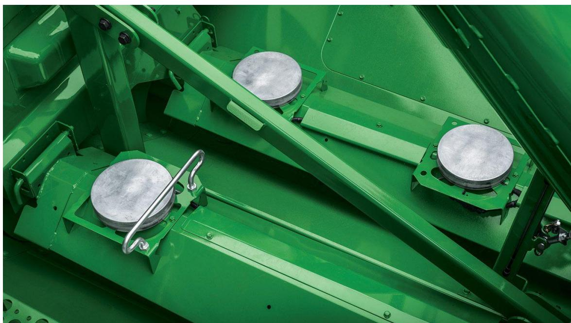
Slika 4. John Deere senzori mase (Izvor: <https://www.martindeerline.com/blog/john-deere-activeyield--active-calibration--8357> )
