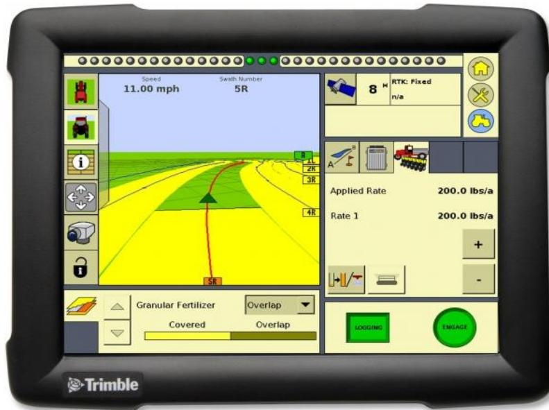
Slika 14. Trimble navigacijski terminal (Izvor: <https://agriculture.trimble.com/solutions/guidance-steering> )
