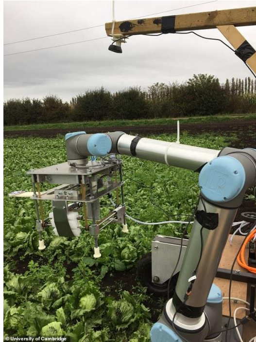
Slika 16. Vegebot u radu ( https://www.agri-tech-e.co.uk/robot-uses-machine-learning-to-harvest-lettuce%E2%80%A8/ )
