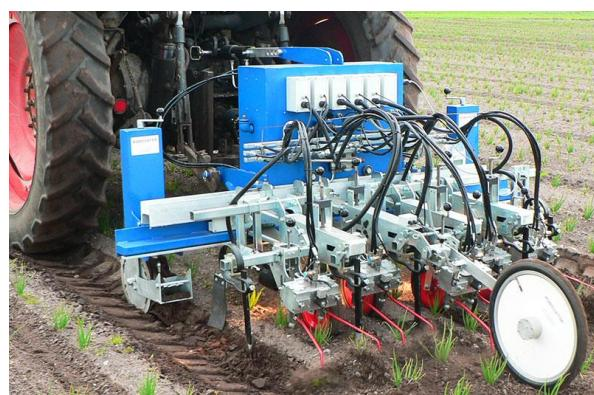
Slika 12. Robovator u povrćarskoj proizvodnji ( Izvor: <https://www.visionweeding.com/robovator-mechanical/>)
