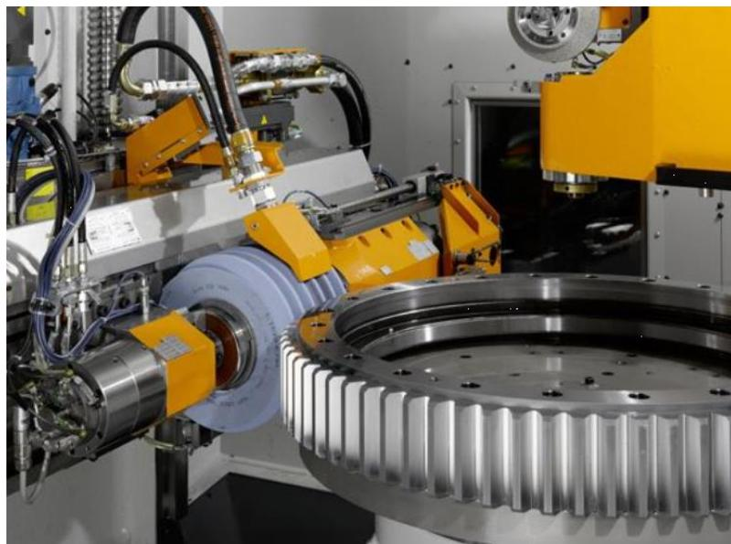
Slika 24. Precizno brušenje zupčanika (Izvor: <http://hr.lemn-machining.nl/Content/ue/net/upload1/Other/134329/6361428886624032468094443.png>)
