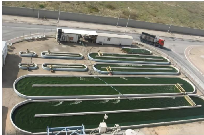
FIGURE 6: Open microalgae cultivation system
