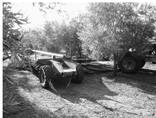
Figure 6. Rolling canvas for high density olive orchards
