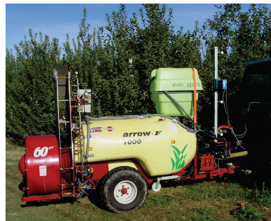
Figure 3 Ultrasonic and LIDAR sensors equipped air assistance sprayer [40]
