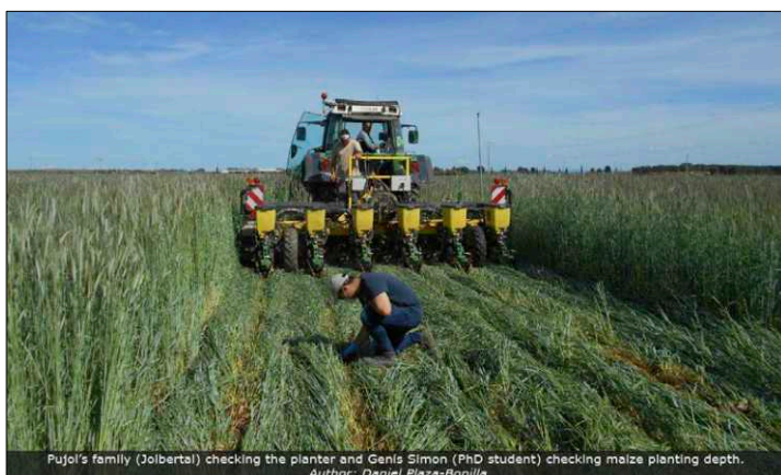
Figure 1. Soybean and maize planting green on rye cover crop in an on-farm sprinkler-irrigated cropping systems experiment located in Sucs (Lleida, Spain) in the framework of the ERA-NET project LegumeGap ( www.legumegap.eu ). Above: individual hydraulic roller-crimpers (ZRX Plus – With Integral row cleaner from Underground Ag Co, Dawn®, Sycamore, IL, USA) are attached to the different no-till row units. Additional weight was added by Jolbertal SL (collaborating farmers) to assure enough soil penetration under harsh conditions. Below: a proper planting depth and rye mulch management requires careful check.
