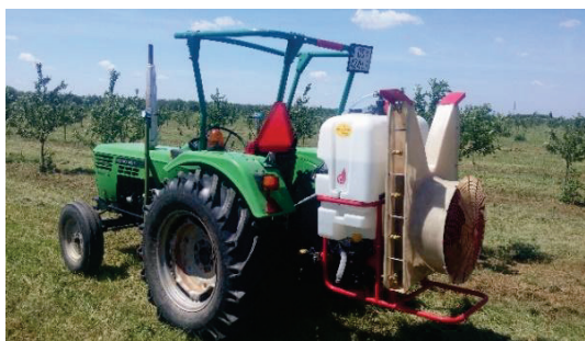
Figure 1 Air assisted sprayer Agromehanika AGP 200 ENU
