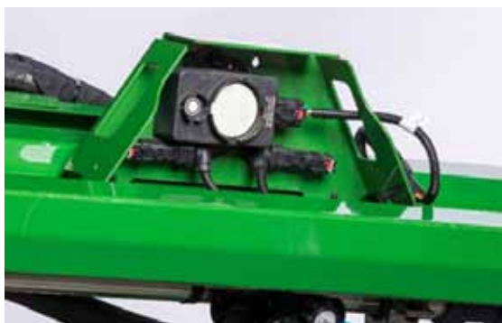
Slika 10. John Deere BoomTrac Pro senzor (Izvor: https://www.plattevalleyequipment.com/blog-news/sprayer-performance-upgrade-kits/ )
