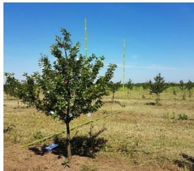
Slika 3. Vertikalno i horizontalno nosači filter papirića Figure 3. Vertical and horizontal collectors for filter papers
