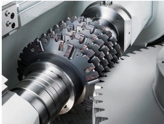
Slika 24. Izrada zupčanika odvalnim glodalom (Izvor: https://s-media-cache-ak0.pinimg.com/originals/bd/44/30/bd4430dce5ac3254724de45e64bb7d7e.jpg )
