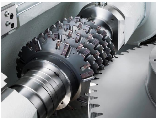
Slika 24. Izrada zupčanika odvalnim glodalom (Izvor: https://s-media-cache-ak0.pinimg.com/originals/bd/44/30/bd4430dce5ac3254724de45e64bb7d7e.jpg )
