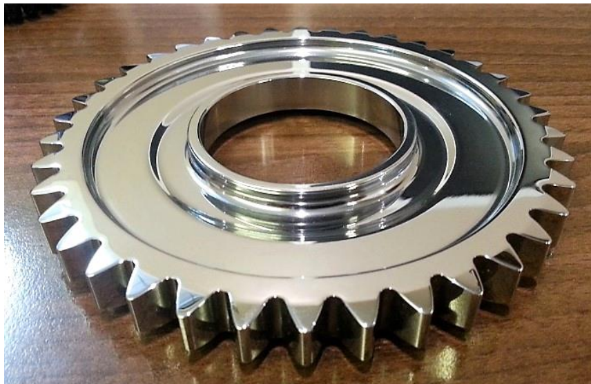
Slika 38. Polirani zupčanik (Izvor: http://www.yorkshire-polishing.co.uk/image-gallery )
