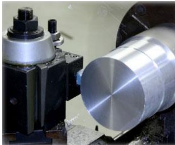
Slika. 3. Tokarenje aluminijске legure ( http://lesmillerdesigns.com/machining.html )
