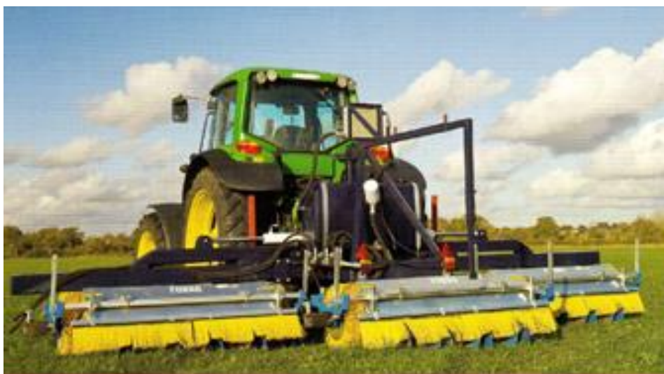
Slika 7. Četkasti kultivator (Izvor: http://www.byeengineering.co.uk/triple-brush-hoe.php )
