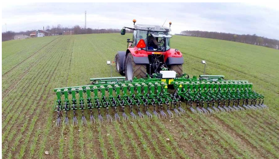
Slika 6. Drljača pljevilica (Izvor: https://www.google.com/search?biw=1600&bih=757&tbm=isch&s )
