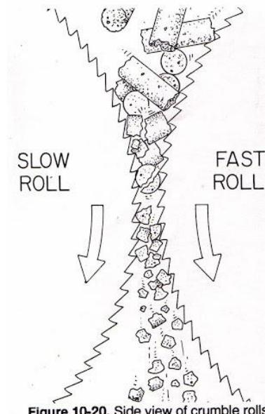
**Figure 10-20.** Side view of crumble rolls.
