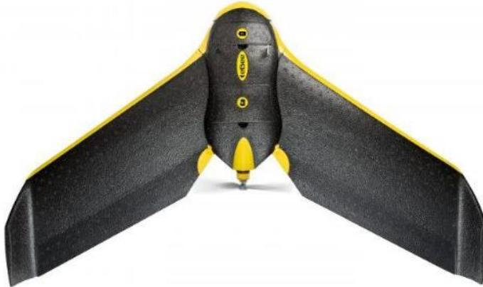
Slika 14. Bespilotni zrakoplov eBee Sensefly <https://www.sensefly.com/drone/ebee-plus-survey-drone/>)
