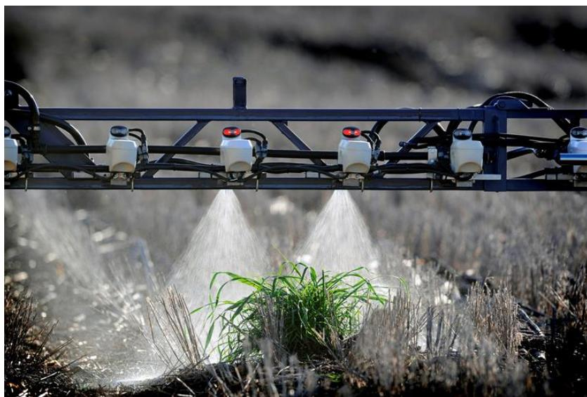
Slika 7. Prskalica opremljena senzorima korova (Izvor: <https://www.weedsmart.org.au>)
