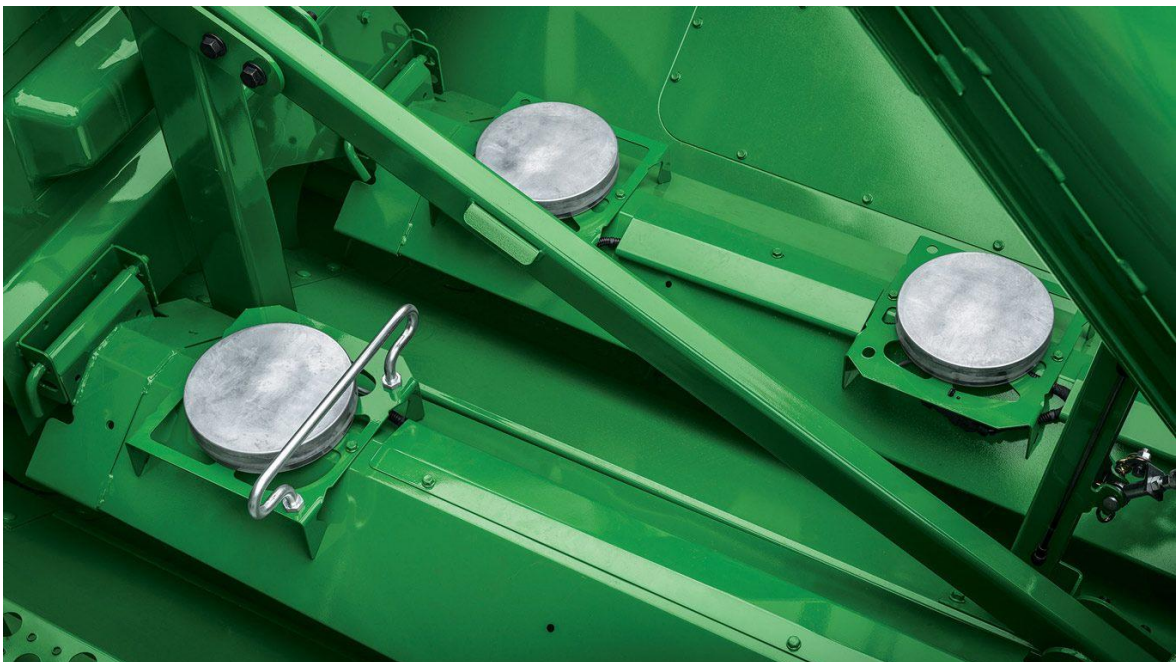
Slika 4. John Deere senzori mase (Izvor: https://www.martindeerline.com/blog/john-deere-activeyield--active-calibration--8357 )
