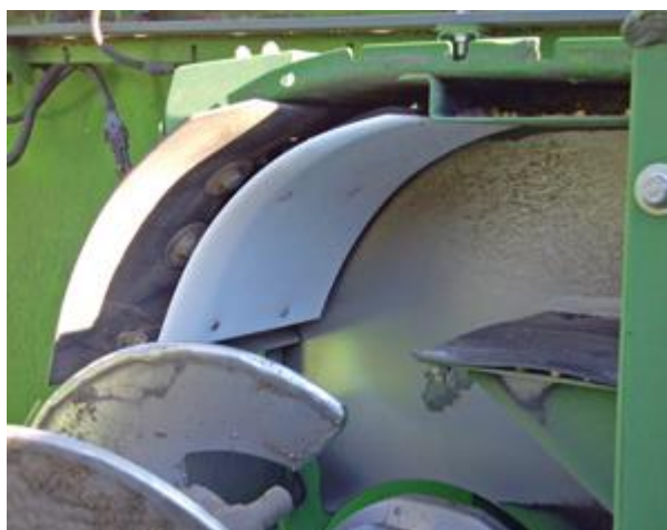
Slika 3. John Deere udarne senzora (Izvor: https://www.maywes.com/products/mass-seed-flow-sensor-impact-plate-8-1-4-x-12-1-2-x-1-8-thick-kit )
