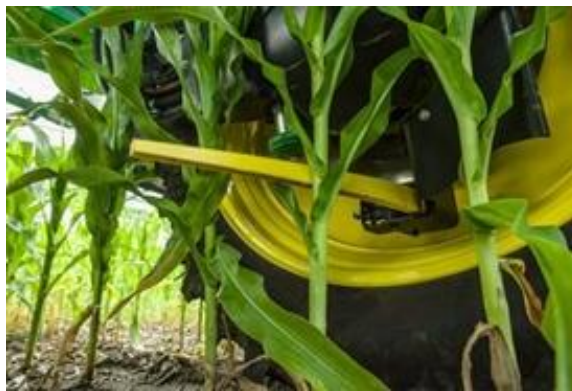
Slika 35. Mehaničko osjetilo za praćenje redova John Deerovog sustava RowSense (Izvor: https://www.evergladesfarmequipment.com/john-deere/agriculture-equipment/precision-agriculture/autotracc%E2%84%A2-rowsense%E2%84%A2/ )
