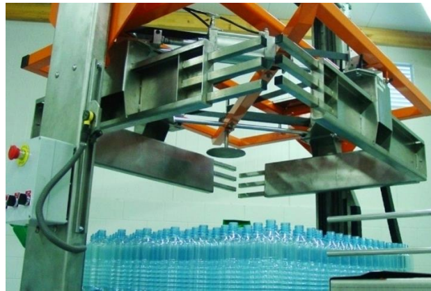
Slika 16. Depaletizator palete boca (Izvor: https://www.scottphs.com/products/depalletizers/ )
