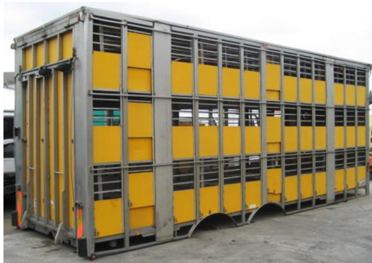
Slika 25. Kontejner za transport živih životinja (Izvor: https://www.truck1.eu/swap-bodies-containers/pioger-et-fils-livestock-transporter-cargo-a687705.html )
