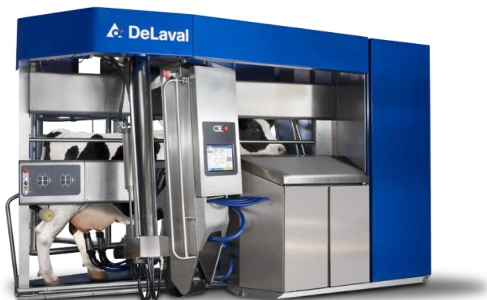
Slika 6. DeLaval automatski muzni sustav (izvor: <https://www.delaval.com/en-us/explore-our-farm-solutions/milking/delaval-vms-series/delaval-vms-your-way/> )
