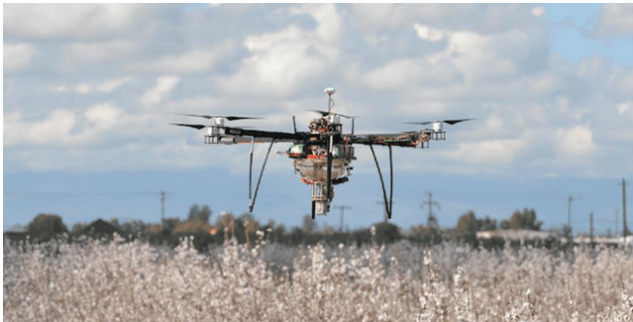
Slika 5. Oprašivanje voćaka iz zraka dronom (Izvor: https://fruitgrowersnews.com/article/new-york-invests-drone-pollination/ )
