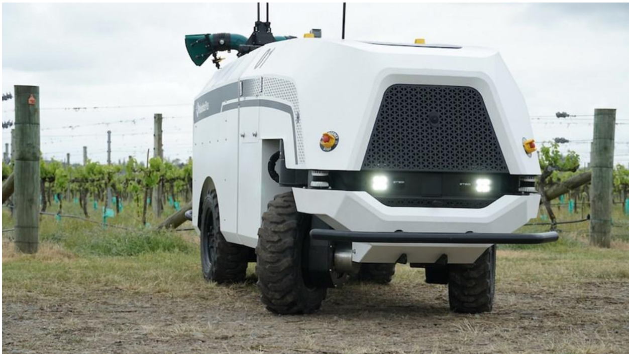
Slika 14. Autonomna modularna platforma za voćnjake i vinograde ( Izvor: https://www.theengineer.co.uk/content/news/robotics-plus-unveils-ugv-for-agriculture/ )
