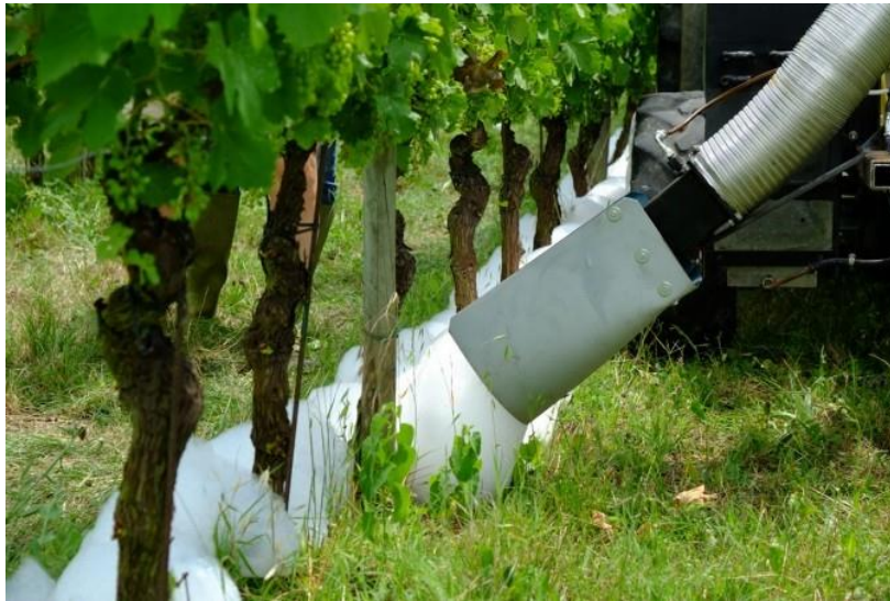
Slika 10. Ekološka kontrola korova zagrijanom pjenom (Izvor: https://en.tecnovict.com/ecological-thermal-weeding-system-with-hot-foam/ )
