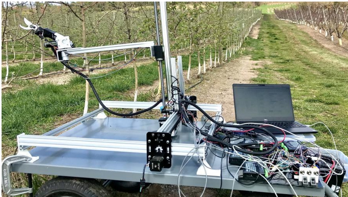
Slika 19. Robotski rezač Sveučilišta Penn State (Izvor: https://www.growingproduce.com/fruits/robotic-pruner-ready-to-cut-down-production-problems-in-apple-orchards/ )
