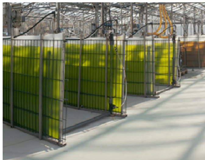
FIGURE 8: Photobioreactors in the form of horizontally placed tubes, vertical flat panels and lyophilized biomass of microalgae
