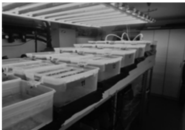
Figure 2. Lighting with GroLux lamps
