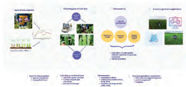
Picture 1. Workflow for detection and evaluation of environmental stress in crops using proximal sensing methods for precise agricultural management decisions
