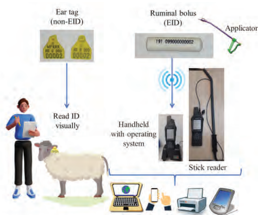
Figure 1. How application of electronic identification (EID) works in small ruminants
