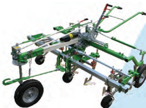
Figure 1. Newly developed inter-row cultivator
