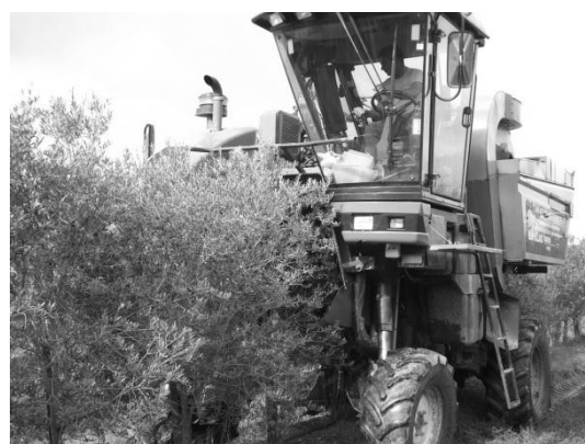
Figure 8. Overrow harvester for hedgerow olive orchards
