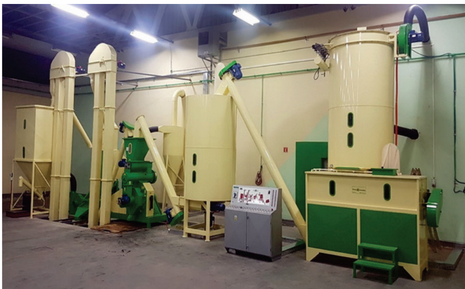
Slika 1. Postrojenje za proizvodnju agropeleta (Izvor: https://www.peletmetalac.com/ ) Figure 1 Facility for agro pellet production (Source: https://www.peletmetalac.com/ )
