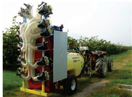
Figure 5 CIS air assistance sprayer [25]
