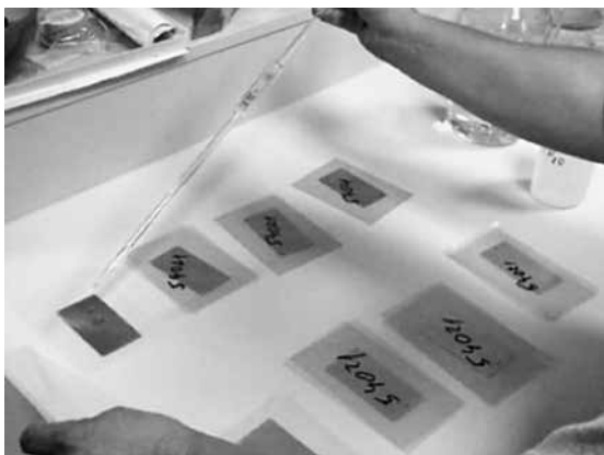
Figure 3 Applying drops of deionized water to the test samples
