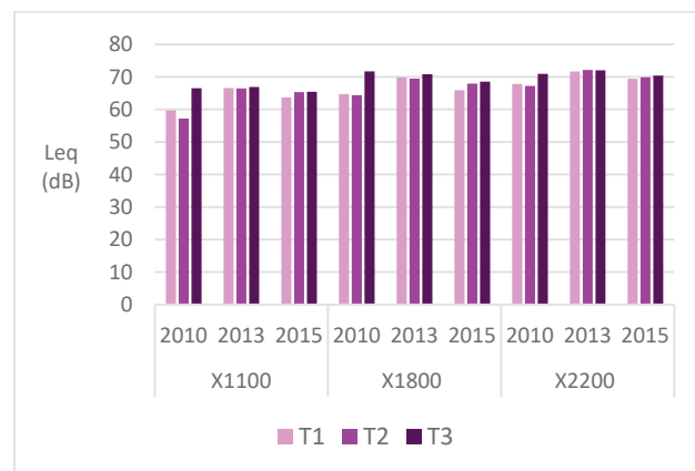
Figure 1 Comparative overview of the mean value of interior noise at a stationary position
