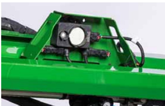
Slika 10. John Deere BoomTrac Pro senzor (Izvor: https://www.plattevalleyequipment.com/blog-news/sprayer-performance-upgrade-kits/ )
