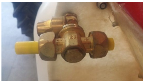
Slika 2. Lechler ITR 8002 i TR 8002 mlaznice Figure 2. Lechler ITR 8002 and TR 8002 nozzles
