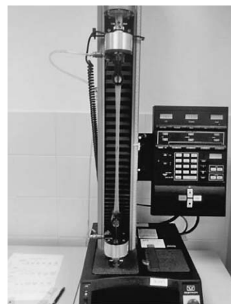
Figure 3 Tensile tester used for measuring the film tear strength
