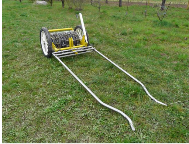
Photo 3. Double traction shafts in front of the roller-cutter for hitching a single horse
