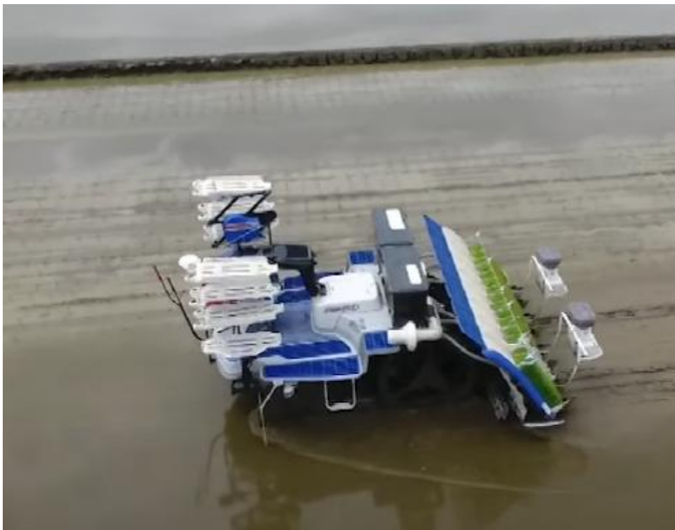
Slika 15. Autonomna sadilica riže (Izvor: https://discoveragriculture.com/ )
