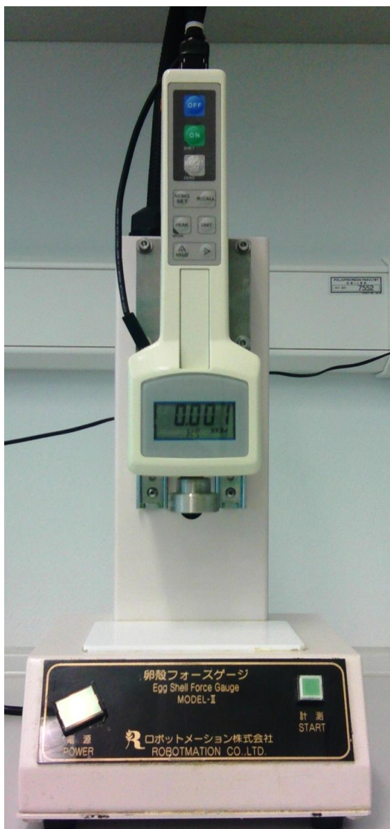
Slika 9. Egg Shell Force Gauge Model – II
