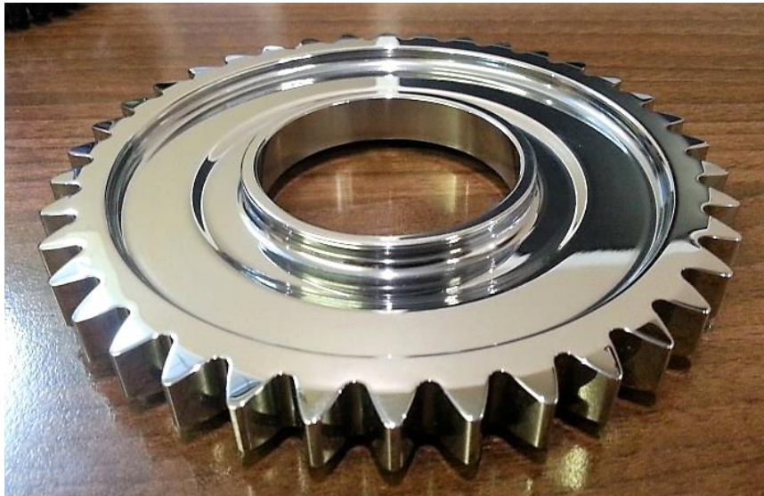
Slika 38. Polirani zupčanik (Izvor: http://www.yorkshire-polishing.co.uk/image-gallery )
