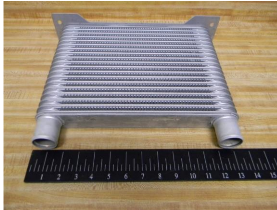
Slika 21. Hladnjak zraka izrađen od limova aluminijske legure ( http://www.ebay.com/itm/New-John-Deere-4066M-Tractor-Turbo-Diesel-Intercooler-LVA17534-TRAD-Inter-Cooler-/151502744419 )
