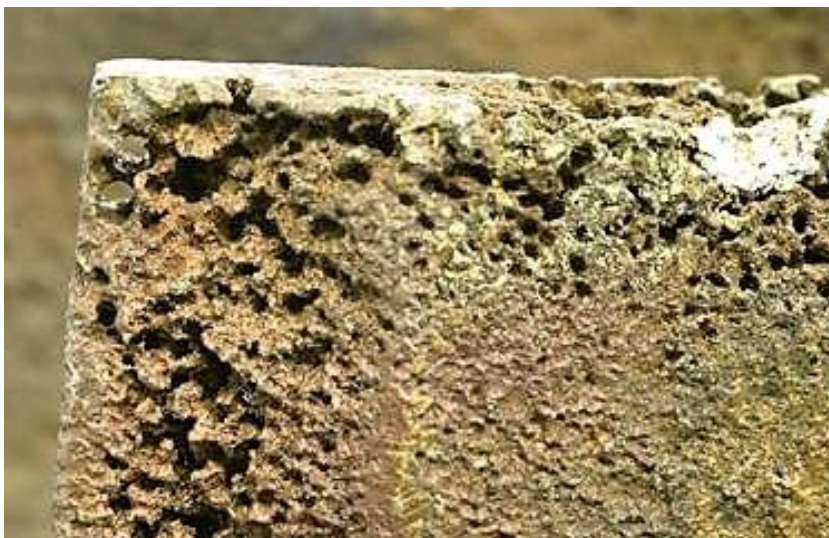
Slika 13. Trošenje tibokorozijom (Izvor: https://www.southampton.ac.uk/engineering/research/facilities/360/nCATS_facility/tribocorrosion.page )
