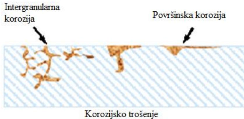
Slika 15. Intergranularna korozija i površinska korozija (Izvor: [https://www.jgs-nitriding.com/images/Content\\_Images/Corrosive\\_Wear.png](https://www.jgs-nitriding.com/images/Content_Images/Corrosive_Wear.png))
