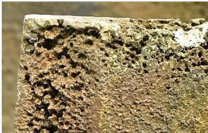
Slika 13. Trošenje tibokorozijom (Izvor: [https://www.southampton.ac.uk/engineering/research/facilities/360/nCATS\\_facility/tribocorrosion.page](https://www.southampton.ac.uk/engineering/research/facilities/360/nCATS_facility/tribocorrosion.page))
