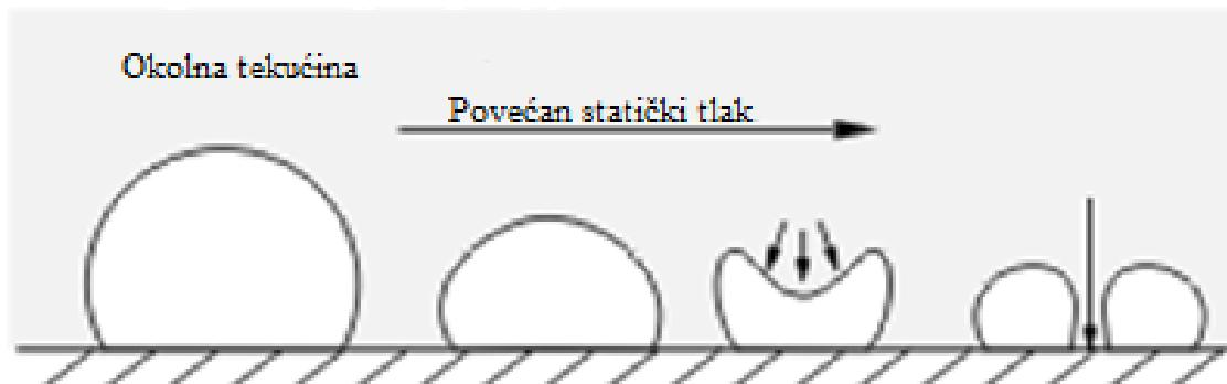
Slika 16. Shema kavitacijskog trošenja (Izvor: [https://en.wikipedia.org/wiki/Cavitation#/media/File:Cavitation\\_bubble\\_implosion.png](https://en.wikipedia.org/wiki/Cavitation#/media/File:Cavitation_bubble_implosion.png))
