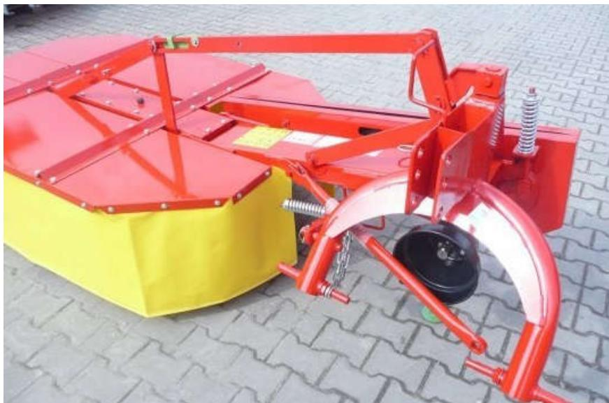
Slika 6. Kosilica-gnječilica,,SIP SIL VERCUT DISC 270 S RC"
