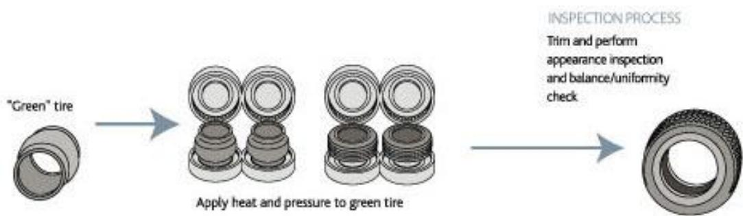
Slika 11. Očvršćivanje i inspekcija (Izvor: <http://fleetsolution-me.com/en/Pages/Tyre-Manufacturing> )
