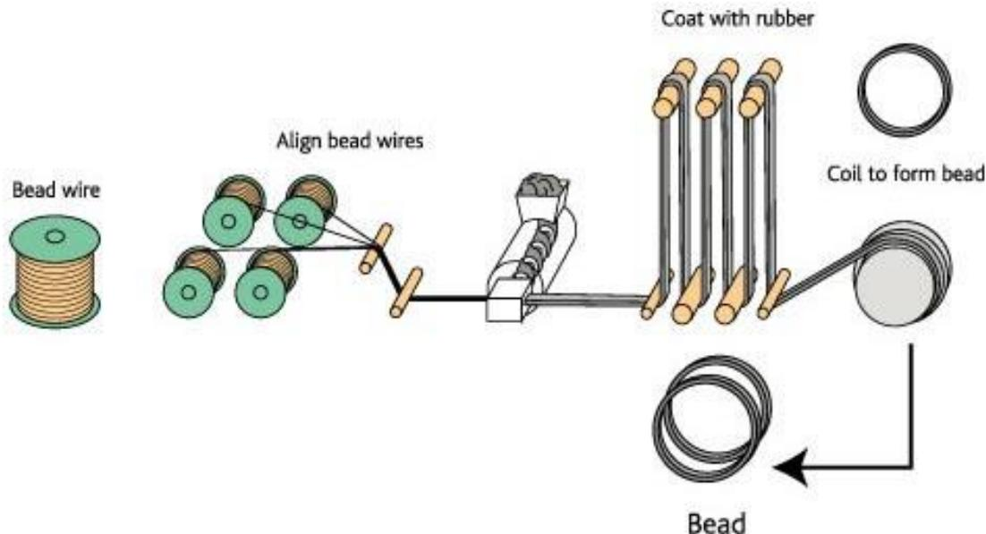
Slika 9. Postupak izrade perli (Izvor: <http://fleetsolution-mea.com/en/Pages/Tyre-Manufacturing> )
