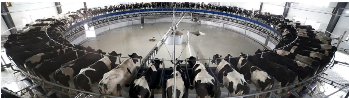
Slika 1. Rotacijsko izmuzište ( https://unfocused.me/2016/10/26/how-much-milk-can-a-cow-hold/ )
