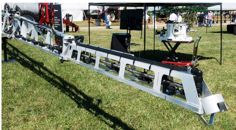
Slika 25. Aluminijске grane prskalice u zaštiti bilja ( https://www.stahly.com/aluminum-booms.php )
