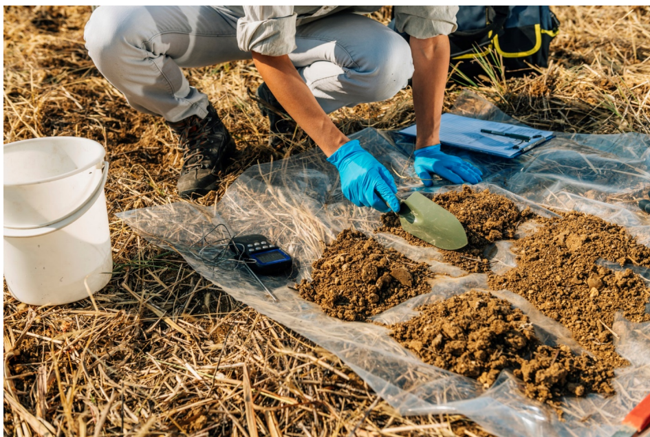
Slika 4. „Četvrtanje“ uzorka (Izvor: https://www.pivotandgrow.com/case/weather-plays-key-role-in-micro-organism-growth/ )
