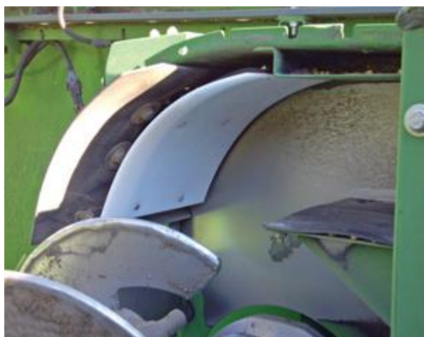
Slika 3. John Deere udarni senzor (Izvor: https://www.maywes.com/products/mass-seed-flow-sensor-impact-plate-8-1-4-x-12-1-2-x-1-8-thick-kit )
