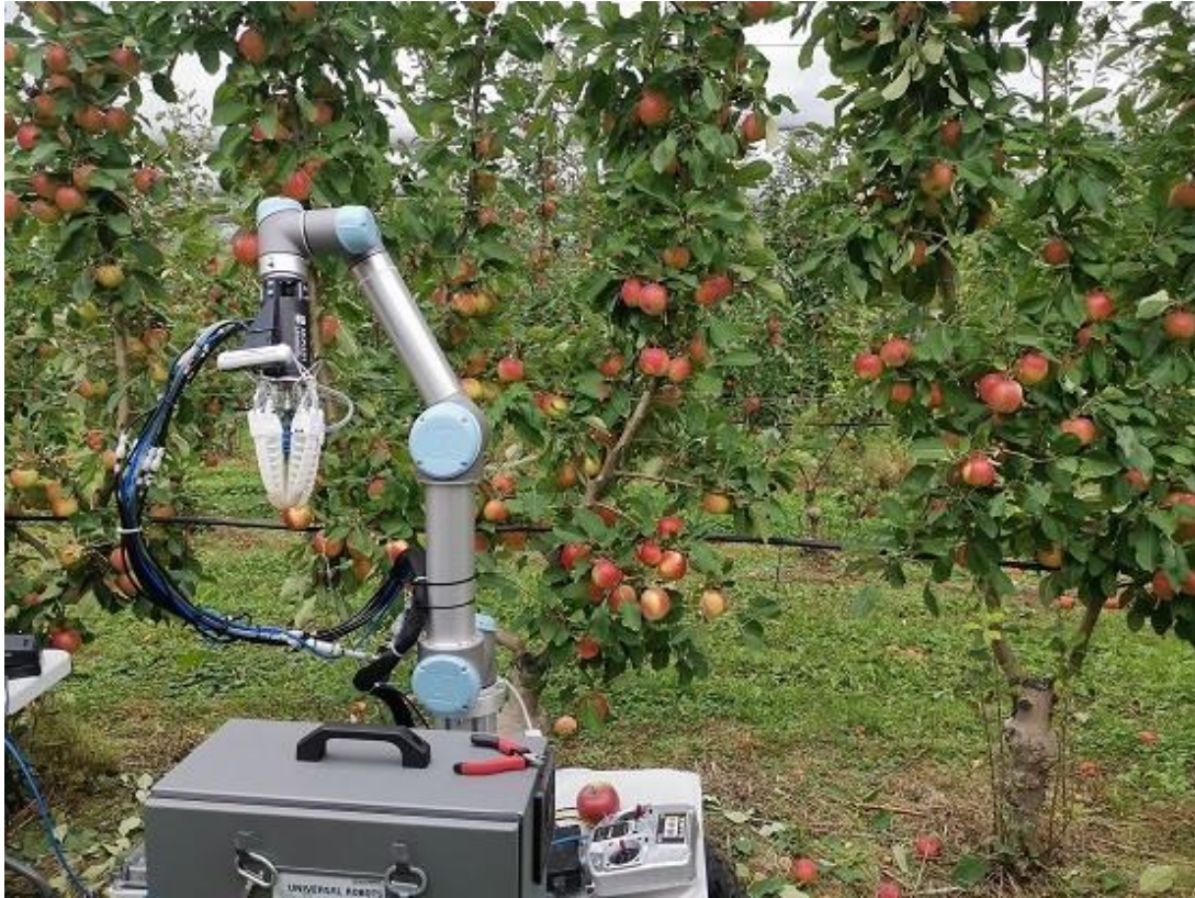
Slika 21. Harvester 3 robot u radu ( https://newatlas.com/robotics/apple-harvesting-robot-fresh-seven-seconds/ )
