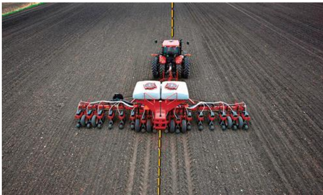
Slika 54. TrueGuide pasivno reduciranje zanošenja priključka, proizvođač Case (Izvor: https://www.caseih.com/northamerica/en-us/products/advanced-farming-systems/auto-guidance/additional-steering-solutions )
