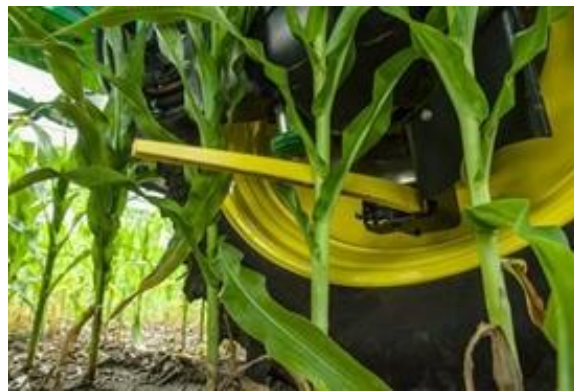
Slika 35. Mehaničko osjetilo za praćenje redova John Deerovog sustava RowSense (Izvor: https://www.evergladesfarmequipment.com/john-deere/agriculture-equipment/precision-agriculture/autotractor%E2%84%A2-rowsense%E2%84%A2/ )
