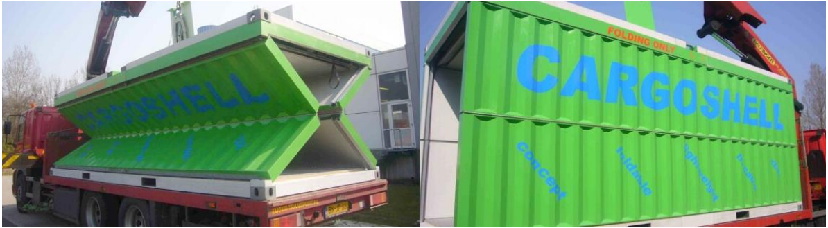
Slika 24. Sklopivi kontejner (Izvor: https://newatlas.com/the-cargoshell-ingenuous-collapsible-replacement-for-the-standard-shipping-container/13736/ )
