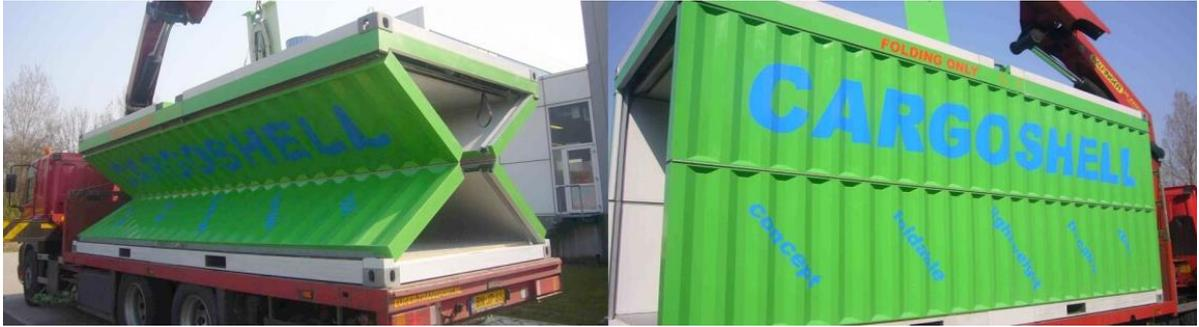
Slika 24. Sklopivi kontejner (Izvor: <https://newatlas.com/the-cargoshell-ingenuous-collapsible-replacement-for-the-standard-shipping-container/13736/>)
