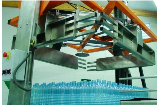
Slika 16. Depaletizator palete boca (Izvor: https://www.scottphs.com/products/depalletizers/ )
