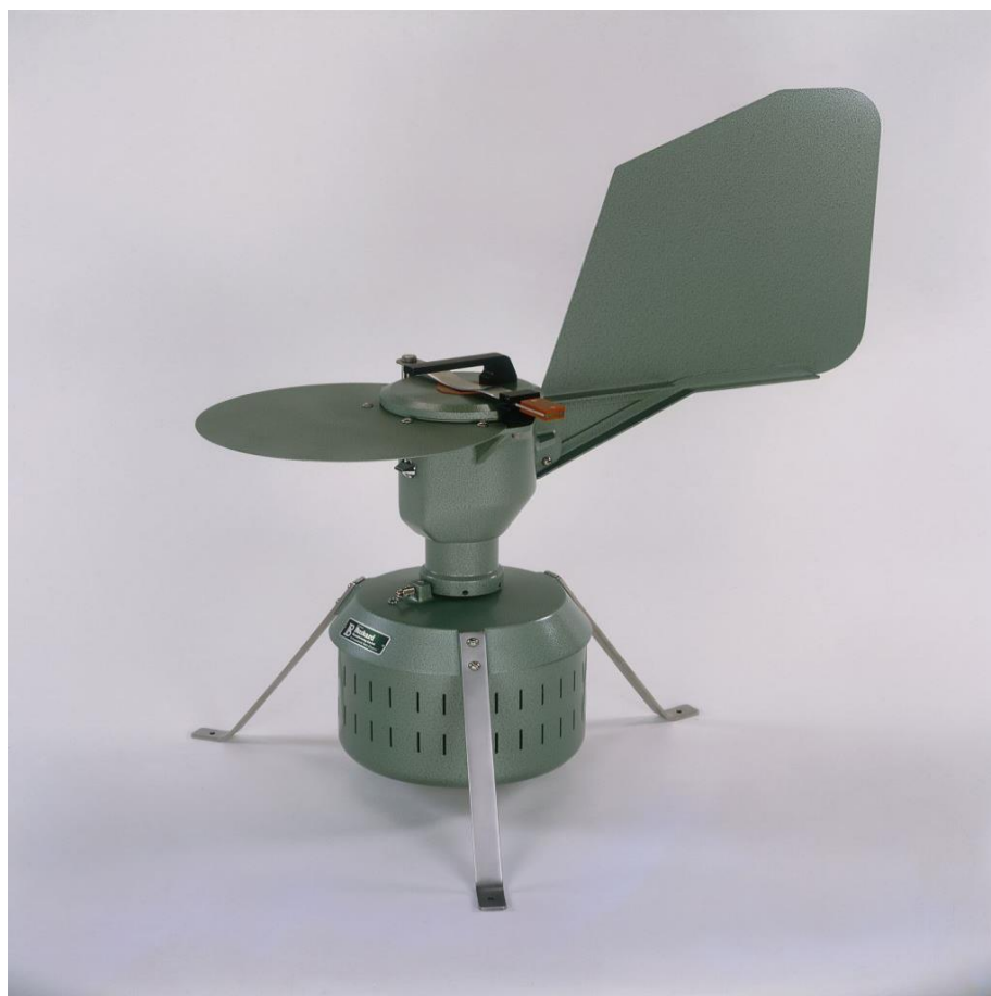
Slika 5. Burkard 7day volumetric spore trap (Izvor: http://burkard.co.uk/product/7-day-recording-volumetric-spore-trap/ )
